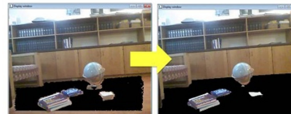
Step 2. This clustering method is based on the similarities of the shape, colors and spatial distance between neighboring pixels.
