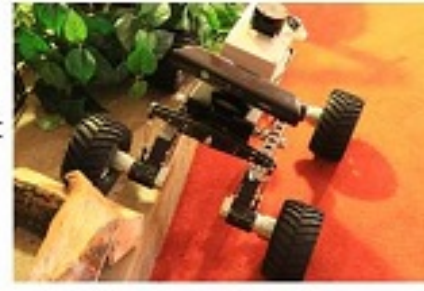
Our robot, equipped with Laser Scanner (top) and Kinect RGBD sensor (front)
