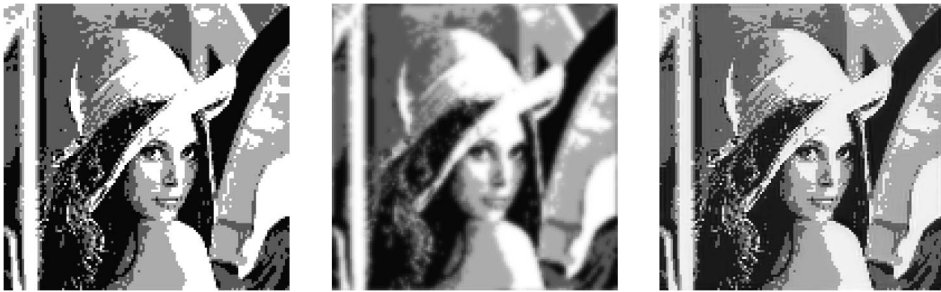
Fig. 4. Blind deconvolution result for a 2-bit image, no noise. True image (left); blurred image (middle); estimated true image (right), ISNR = 13.66 dB.
