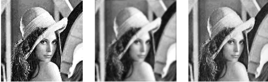
Fig. 6. Blind deconvolution result for a 4-bit image, no noise. True image (left); blurred image (middle); estimated true image (right), ISNR = 6.12 dB.
