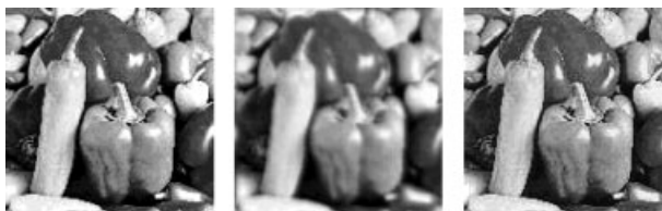
Figure 9. Deconvolution result for the SPR PSF, L = 16 . ISNR = 38.80 dB.
