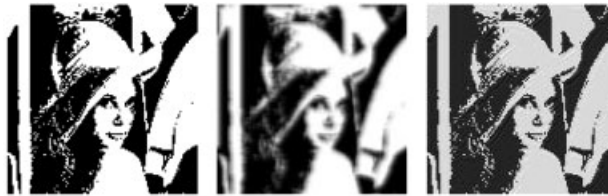
Figure 11. Deconvolution result for the non-SPR PSF, L = 2 . ISNR = 40.51 dB.
