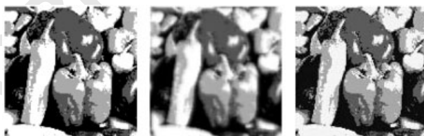
Figure 7. Deconvolution result for the SPR PSF, L = 4 . ISNR = 45.30 dB.
